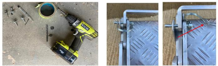
Place the masking tape on the camper chassis below the entrance door. Position the bracket under the door (over the tape). Make sure the bracket does not obstruct any door movement when the door is opening or closing. Mark the four holes on to the tape below the door.
