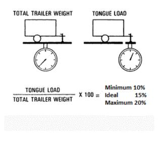
The drawing to the left illustrates the proper weight distribution for loading a trailer. Use the Weigh Station scale to achieve a minimum of 10% to a maximum of 20% of the total trailer weight of the trailer as tongue weight. A proportional tongue weight provides the best handling for addressing trailer sway. Reasonable driving speeds and proper tire inflation are equally important.
