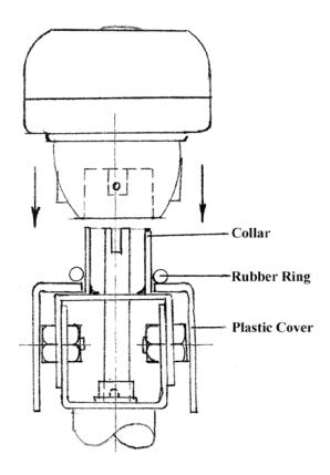
Rieco-Titan Jacks- The drive pin in the jackpost must be knocked out. The old bushing and washer must be replaced with a new steel bushing. Install new 5/32" drive pin so that it is equally protruding on each side to fit inside the drive tube collar. Clean gearbox with cloth or paper towel. No solvents.
