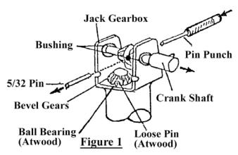
5. Lift the horizontal bevel gear off the jackpost drive pin. Follow instructions on figure #2 for the type of jack you are converting. Clean gearbox of grease, using cloth or paper towel.
