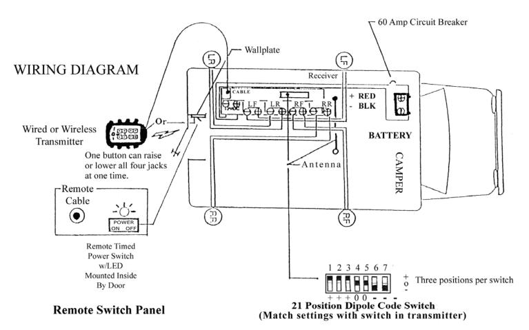
IN ORDER TO OPERATE THIS ELECTRIC JACK SYSTEM, IT IS NECESSARY TO INSTALL A HEAVY DUTY MARINE/RV BATTERY WITH PROVISION TO KEEP THE BATTERY CHARGED. LOCATE IT IN A SEPARATE SITE, BUT NEAR THE RECEIVER.
