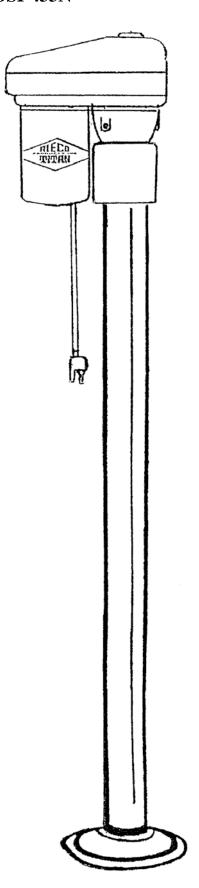
CAUTION !!! If your jacks are ball screw type, with tube welded to side of gear box, make sure your camper is on your truck or supported on blocks, so that the camper cannot tip over while you are working on this conversion!
